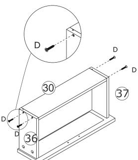
Use screw D to connect panel 30 to panel 36 and 37.
