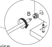
Connect panel 38 to panel 36 and 37, and clockwise rotate eccentric wheel B to lock it.
