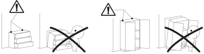
Install anti-tipping device as shown.
