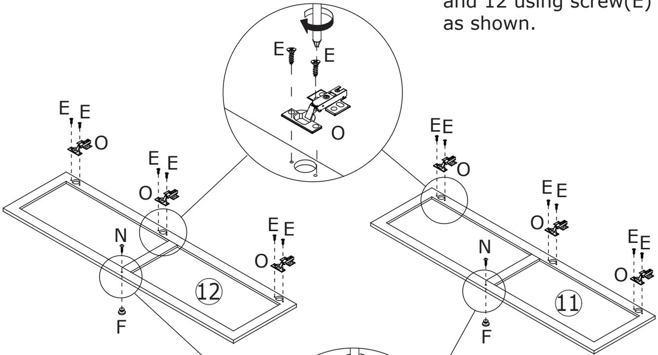
Fix knob(F) using screw(N) as shown.
