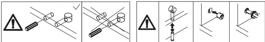
Attach plate 10 to plate 3,9 and 16 with wooden dowel(C), insert cam lock(B) into plate 3,9,16 and turn clockwise to tighten as shown.
