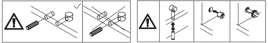
Attach plate 3 to plate 9 with wooden dowel(C) at first; attach plate 3 to plate 8, insert cam lock(B) into plate 8,9 and turn clockwise to tighten as shown.
