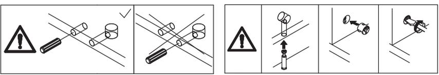
Connect the two assembled components using wooden dowel(C), insert cam lock(B) into plate 3,16 and turn clockwise to tighten as shown.
