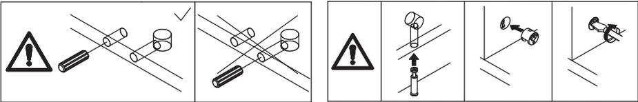
Attach plate 15 to plate 1 and 6 with wooden dowel(C), insert cam lock(B) into plate 1,6 and turn clockwise to tighten as shown.
