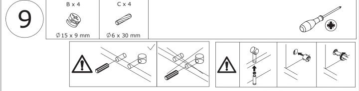
Connect plate 10 and 12 with plate 13 using wooden dowel(C), insert cam lock(B) into plate 13 and turn clockwise to tighten as shown.
