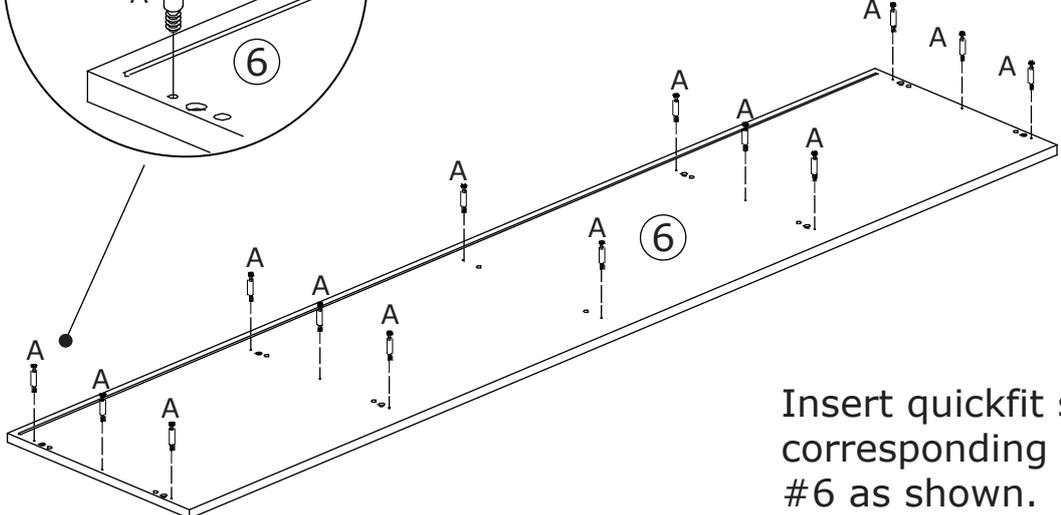
Insert quickfit screw(A) into corresponding holes in plate #6 as shown.
