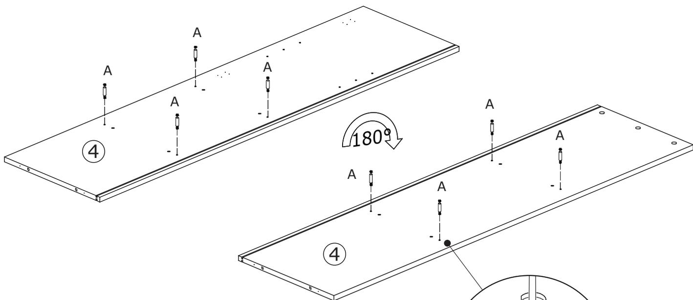
Insert quickfit screw(A) into corresponding holes in both sides of plate #4 and #5 as shown.
