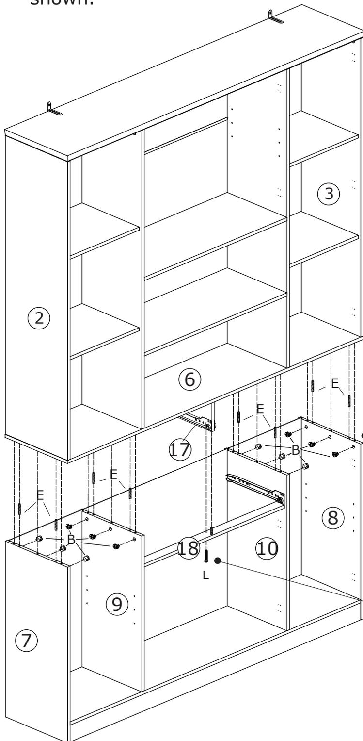
Fix plate #17 with plate #18 using screw(L) as shown. Requires more than two people to assemble.
