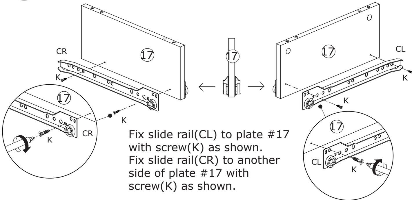
Fix slide rail (CL) to plate #17 with screw (K) as shown. Fix slide rail (CR) to another side of plate #17 with screw (K) as shown.
