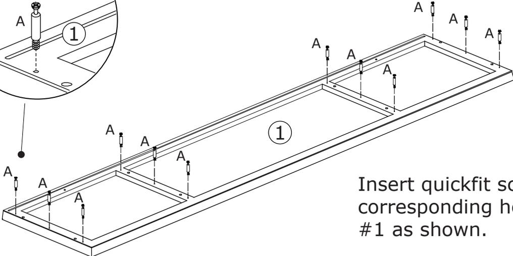
Insert quickfit screw(A) into corresponding holes in plate #1 as shown.
