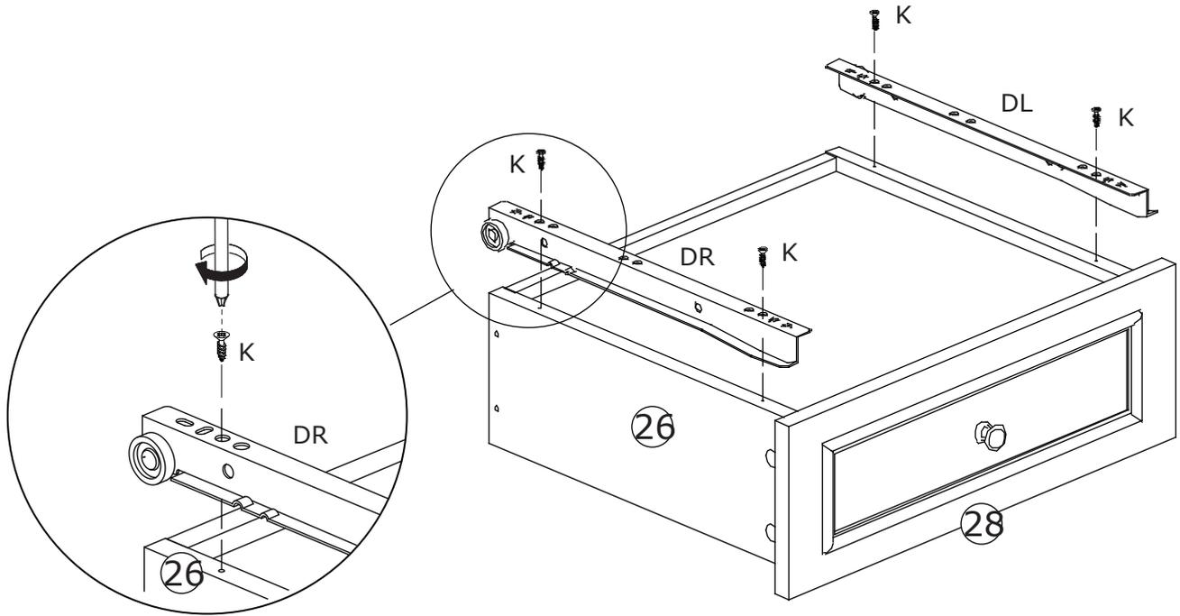
Fix runner(DL) and (DR) to plate #25 and #26 with screw(K) as shown.
