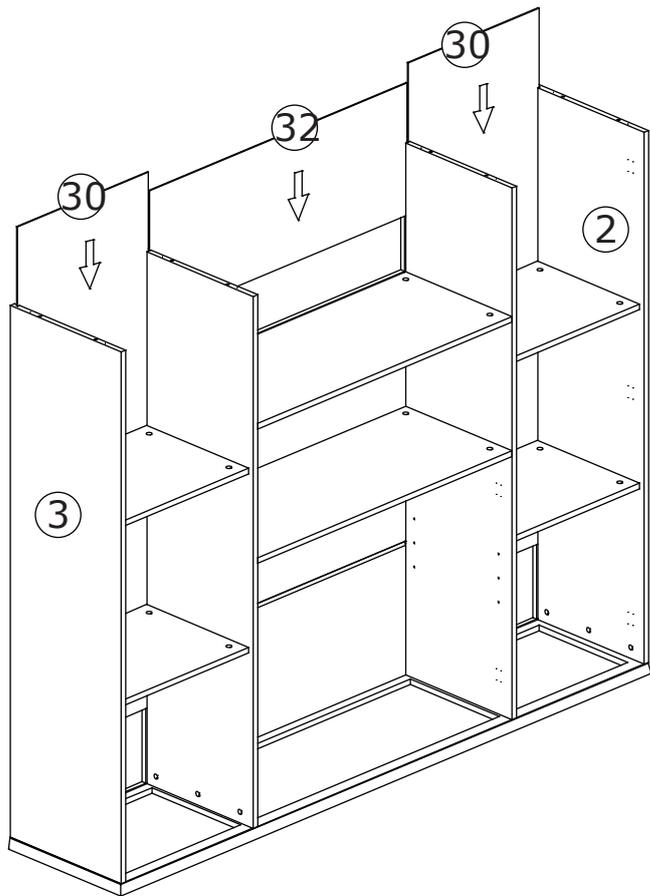
Slide plate #30 and #32 into available grooves at first.
