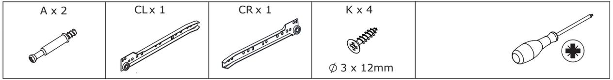
Fix slide rail(CL) and (CR) to plate #9 and #10 respectively using screw(K) as shown. Insert quickfit screw(A) into plate #9 and #10 with a screwdriver as shown.
