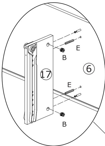
Attach plate #17 to plate #6 with wooden dowel (E), put cam lock (B) into plate #17 and turn clockwise to tighten as shown.
