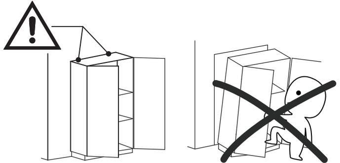
Drill holes on your wall, and install anti-tipping device as shown.
