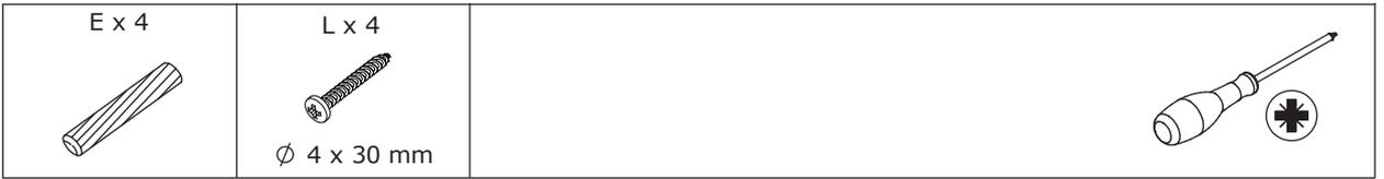
Connect the two components (assembled in step 2 and 4) with wooden dowel (E), then fix with screw (L) as shown.
