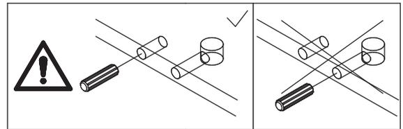
Connect two plate #13 with plate #5 using wooden dowel(E), put cam lock(B) into plate #13, turn clockwise to tighten as shown.
