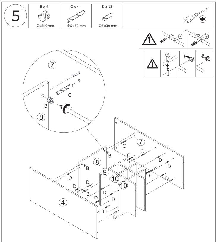
Attach board 4 to board 8,9,10 with short wooden dowel(D) and turn cam locks(B) clockwise to tighten as shown.
