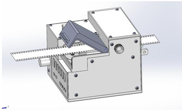
Connect with tape **the waste film** and **the film from the magazine**
