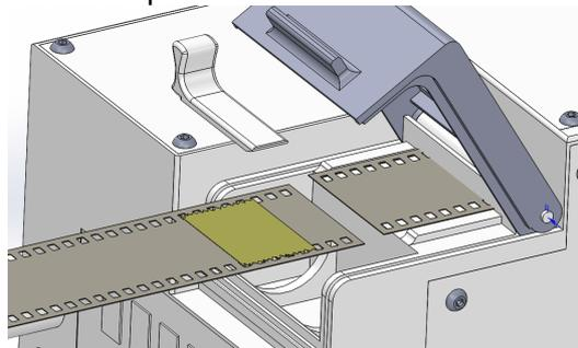
**\*You can ignore STEP 3 and just pull the film from the magazine, going through the film loader from the rear to the front, but you will waste about 5 exposures.**
