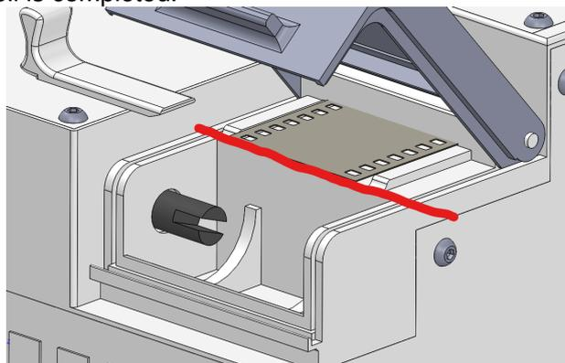
Put another canister into the film loader, close the cover, **press R/S** to start the second roll, and so on.
