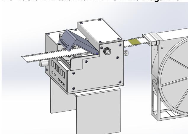
Pull the waste film from the front while attaching the magazine to the film loader, and insert the locking knob
