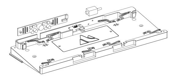
7. Attach the GASKET pad to the interior of the top shell and place the TOP pad on the top shell's projection.
