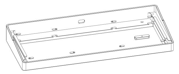
9.According to personal preference, layer the bottom foam and hot-swappable foam inside the baseplate to fill the space (After installing the PCB and satellite axis, stack the PCB, lower pad, soundproofing foam, and positioning plate together, then secure them into the axle body. Connect the ribbon cables, aligning the PCB holes with the silicone grains on the plate spring so that the silicone grains fit into the PCB.)
