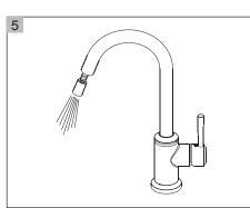
After installation is complete, remove Spray head and rotate handle to the close position. Turn Water Supply Valves on, and check all connections for leak. Flush faucet by running hot and cold water in full position for one minute.
