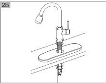
Make sure the O-RING is placed onto the bottom of Base Ring. Install faucet through Deck Plate. From underside sink, put Plastic Washer and Mounting Nut. Position faucet on sink properly and tighten Mounting Nut.
