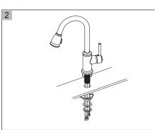
Install without Deck Plate. Make sure the O-RING is placed onto the bottom of Base Ring. Install faucet through hole in sink. From underside sink, put Plastic Washer and Mounting Nut. Position faucet on sink properly and tighten Mounting Nut.
