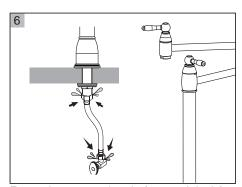
Turn on the water supply to the faucet and check for leaks.
