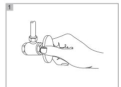
You should clean all the dirts from valve outlets. Turning off the water supply valves. This is usually found near the water meter. If you are replacing an existing faucet, remove the faucet from the sink and clean the sink surface thoroughly.
