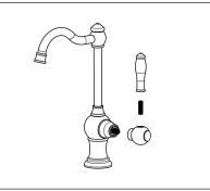
Turn off water and relieve pressure! Detach handle button using a small flathead screwdriver, unscrew set screw using Allen Wrench and take off handle.
