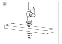
Install without Deck Plate. Make sure the O-RING is placed onto the bottom of Base Ring. Install faucet through hole in sink. From underside sink, put Plastic Washer and Mounting Nut. Position faucet on sink properly and tighten Mounting Nut.
