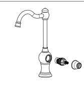
Remove handles. Unscrew Dome Cap counter clockwise by hand. Unscrew Retaining Nut using adjustable wrench, take out cartridge assembly and inspect. Replace parts as necessary. Reassemble parts by reversing steps.
