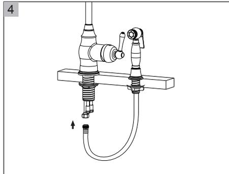
Insert spray hose down through spray seat, then connect the spray hose to the outlet hose at the bottom of the tap and tighten it.
