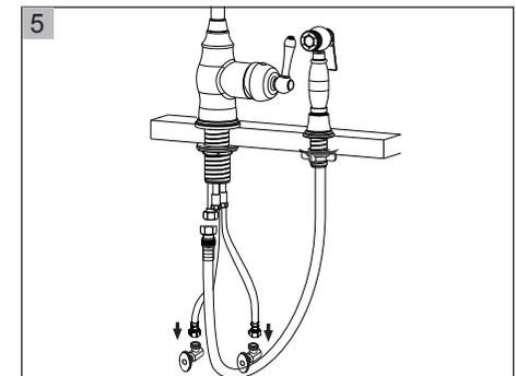
Connect the hot and cold water supply lines of the faucet to the water supply valves.
