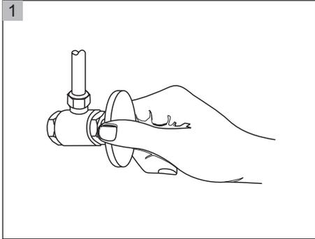
You should clean all the dirt from valve outlets. Turning off the water supply valves. This is usually found near the water meter. If you are replacing an existing faucet, remove the faucet from the sink and clean the sink surface thoroughly.
