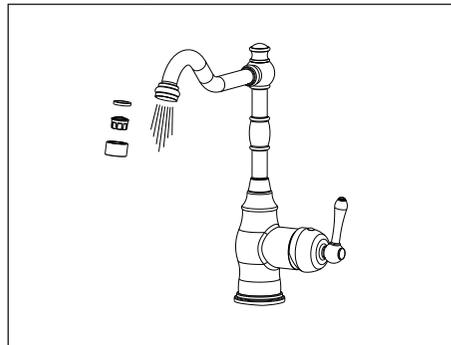
After installation is complete, remove aerator and rotate handle to the closed position. Then turn on the water supply valves, and check all connections for a leak. Turn on your faucet and allow both hot and cold water to run at least one minute each, then Install the Aerator.
