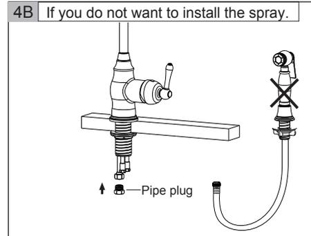
If you do not want to install the spray, please plug and tighten it with the stopper "L".
