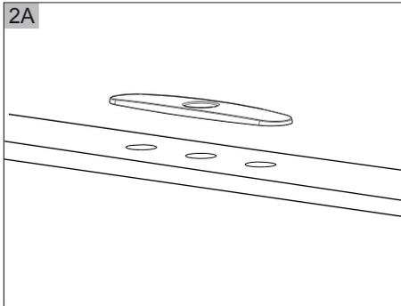
Install with deck plate. Place a bead of plumber's putty between faucet and sink. Place deck plate over the three holes of sink.
