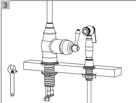
If necessary, tighten screws using an adjustable wrench until the faucet is firmly connected to the sink.
