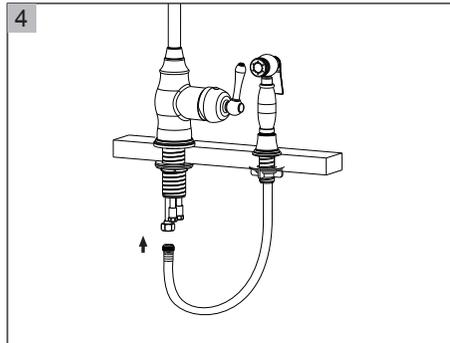
Insert spray hose down through spray seat, then connect the spray hose to the outlet hose at the bottom of the tap and tighten it.
