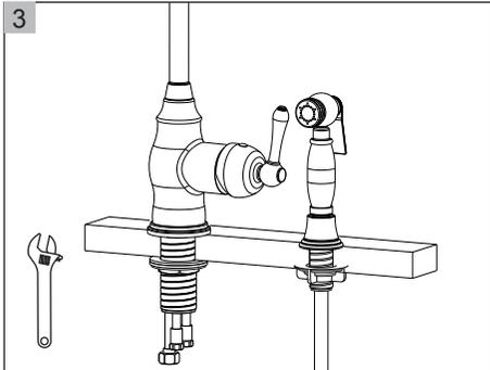
If necessary, tighten screws using an adjustable wrench until the faucet is firmly connected to the sink.
