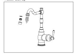
After installation is complete, remove aerator and rotate handle to the closed position. Then turn on the water supply valves, and check all connections for a leak. Turn on your faucet and allow both hot and cold water to run at least one minute each, then Install the Aerator.
