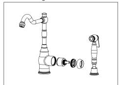
Remove handles. Unscrew Dome Cap counter clockwise by hand. Unscrew Retaining Nut using adjustable wrench, take out cartridge assembly and inspect. Replace parts as necessary. Reassemble parts by reversing steps.
