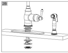
Make sure the O-ring is placed onto the bottom of base ring. Install faucet through deck plate. From underside sink, put plastic Wwasher and mounting nut. Position faucet on sink properly and tighten mounting nut.
