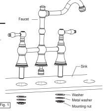
2. Insert spray seat through far right-hand hole on sink. Then tighten mounting nut using adjustable wrench. Insert spray hose down through spray seat, then Joint is installed in the end of the pipe, and tighten it using wrench, then as shown in the figure insert the connector from the body in the middle hole, and attention to whether to whether the installation in place.
