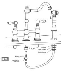
3. Connect spout hot water supply line to the left valve connector. connect Spout cold water supply line to the right valve connector, and connect hot and cold water supply lines to the water supply valves, then tighten Supply line nut.
