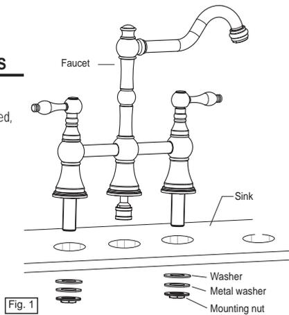
2. Insert spray seat through far right-hand hole on sink. Then tighten mounting nut using adjustable wrench. Insert spray hose down through spray seat, then Joint is installed in the end of the pipe, and tighten it using wrench, then as shown in the figure insert the connector from the body in the middle hole, and attention to whether to whether the installation in place.
