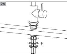
Install without deck plate. Make sure the O-ring is placed onto the bottom of base ring. Install faucet through hole in sink, position faucet on sink properly and tighten the nut from underside of the sink.
