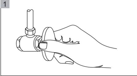
1 Remove any debris from valve outlets. Turning off the water supply valves.
