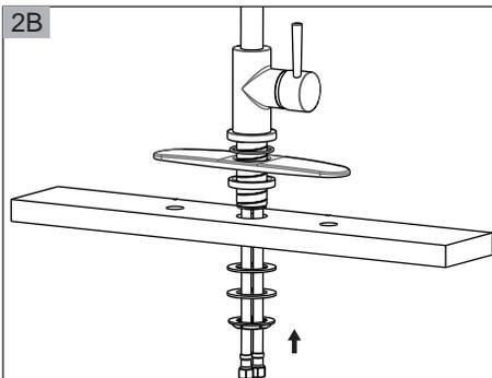
2B Install with deck plate. Position deck plate onto sink. Make sure the O-RING is placed at the bottom of the faucet base. Install faucet through hole in deck plate. From underside of sink, attach mounting assembly. Position faucet on deck plate properly and tighten Mounting Nut.
