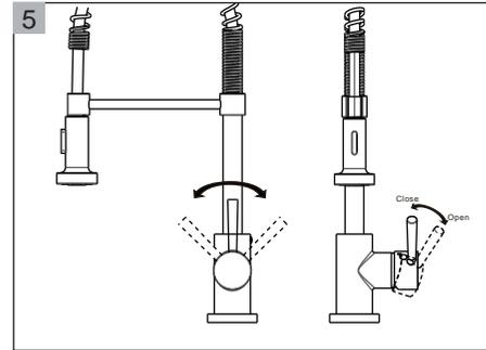
5 Open the valve, then turn the handle according to the sign of C and H on the handle to regulate the temperature of the water. (C=Cold,H=Hot)
