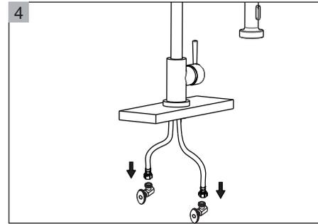
4 Open the water supply valve and flush for about a minute to clear the rubbish left in the pipeline, then turn off the water supply valve, and connect hot and cold water lines of the faucet to the water supply valves.
