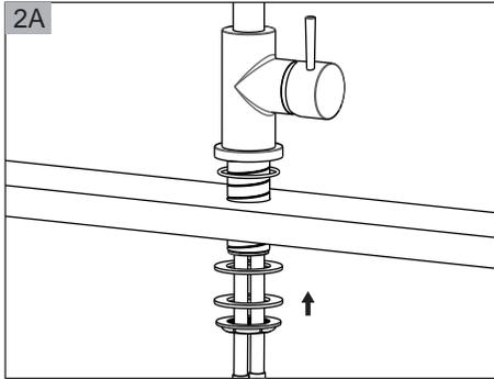
2A Install without deck plate. Make sure the O-ring is placed onto the bottom of base ring. Install faucet through hole in sink, position faucet on sink properly and tighten the nut from underside of the sink.
