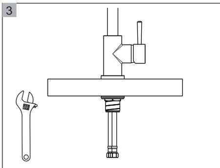
3 If necessary, tighten screws using an adjustable wrench until the faucet is firmly connected to the sink.
