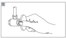
Remove any debris from valve outlets. Turning off the water supply valves.
