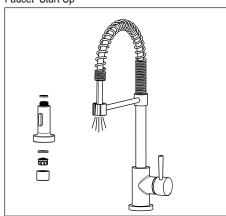
fter installation is complete, remove aerator and rotate
