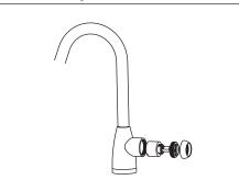
Remove handles. Unscrew dome cap counter clockwise by hand. Unscrew retaining nut using adjustable wrench, take out cartridge assembly and inspect. Replace parts as necessary. Reassemble parts by reversing steps.
