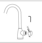
Turn off water and relieve pressure! Detach handle button using a small flathead screwdriver, unscrew set screw using Allen Wrench and take off handle.
