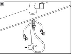
Attach Weights to the pull-out hose using screws at the proper point of the hose. Be noted position of the installation and weights are optional.
