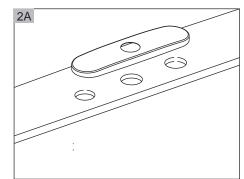
Install with Deck Plate. Place a bead of plumber's putty between faucet and sink. Place Deck Plate over the three holes of sink.
