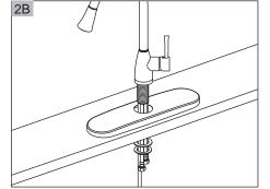
Make sure the O-ring is placed onto the bottom of Base Ring. Install faucet through deck plate. From underside sink, put plastic washer and mounting nut. Position faucet on sink properly and tighten mounting nut.
