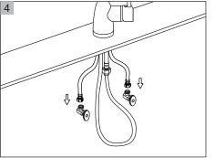
Open the water supply valve and flush for about a minute to clear the rubbish left in the pipeline, then turn off the water supply valve, and connect hot and cold water lines to the water supply valves.
