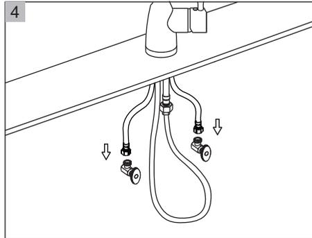
Open the water supply valve and flush for about a minute to clear the rubbish left in the pipeline, then turn off the water supply valve, and connect hot and cold water lines to the water supply valves.
