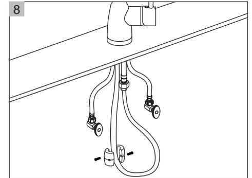
Attach Weights to the pull-out hose using screws at the proper point of the hose. Be noted position of the installation and weights are optional.
