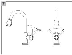
Open the valve, then turn the handle according to the sign of C and H on the handle to regulate the temperature of the water. (C=Cold,H=Hot)
