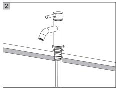
Install without Deck Plate. Make sure the O-RING is placed onto the bottom of Base Ring. Install faucet through hole in sink. From underside sink, put Plastic Washer and Mounting Nut. Position faucet on sink properly and tighten Mounting Nut.
