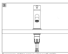
If necessary, tighten screws using a adjustable wrench until the faucet is firmly connected to the sink.
