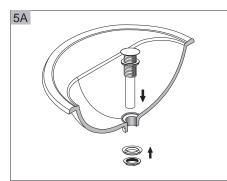
Unscrew Locknut. Make sure the Rubber Washer in the right position under Flange. Insert Pop-up Assembly into Sink drain Hole. From underneath, tighten with Lockset.
