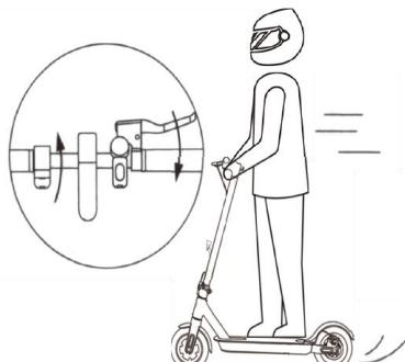
4. Release the accelerator and the kinetic energy recovery system (KERS) initiates automatically to brake slowly; And squeeze the brake lever for a sudden brake.
