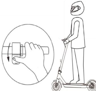
3. When the scooter starts to coast, put both feet on the deck and press the accelerator (the accelerator initiates once the coasting speed exceeds 3mph)
