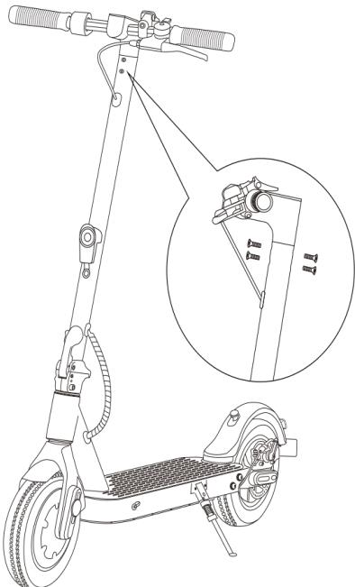
1. Unfold the stem and close the folding latch until you hear a click. Then unfold the kickstand to support the scooter.
