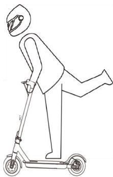
When the scooter starts to coast, put both feet on the deck and press the accelerator (the accelerator initiates once the coasting speed ).
