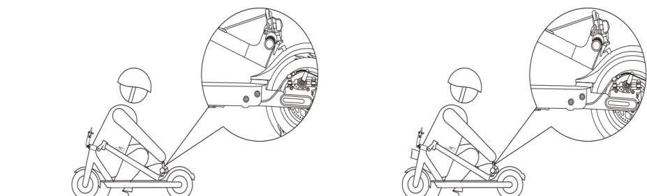
Make sure that the scooter's turned off. To fold, unlock the folding mechanism, and bend the handlebar stem to hook the buckle on the rear fender. To open, press the bell trigger to remove from the buckle, erect the handlebar and lock the folding structure.
