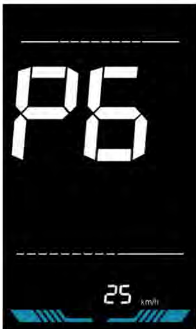
Figure 6-7 Speed limit setting interface
