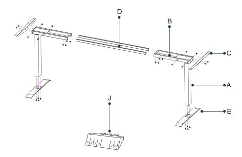
All the above connecting screws use M6 \* 13 screws (G)
