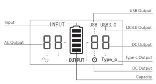
1) How to provide power for DC12V appliances(such as head lamp,fan) with this product? The 5.5mm 12V DC output is plug and play. Plug your appliances to the DC output port to gain power. DC output rated power<120W,Max output<145W.
