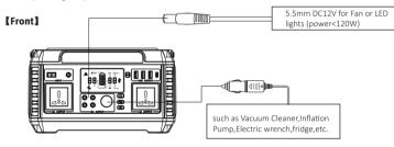
Note: The12V DC output voltage is range between 9V~12.6V, maximum output current is 12A. DC output voltage drops while battery capacity drops due to chemical characteristics of the battery. If your appliance is not built-in input voltage stabilizing function, it may shutdown when input voltage is too low, please unplug your device from the unit in time And please charge the unit in time
