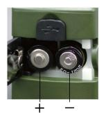
3V-5V battery pack (500mAh-2000mAh) with micro USB connector inserts Micro USB Port on L800.
