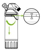
Align the triangle marks, then install the filter body and rotate 90 degrees clockwise to the locking mark.
