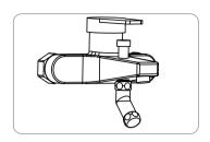
Discharge the filter cartridge, and attach the filter head to the connector and tighten by wrench.
