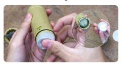
Put a new PP screen in water inlet cover. Screw cover back.
