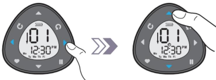
Press "◀" or "▶" to select the channel number. The selected one will be flashing.
