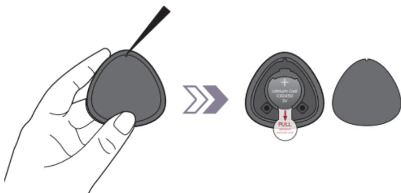
3 Remove the insulating sheet.
