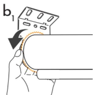
Rotate the gear by 45° vigorously.
