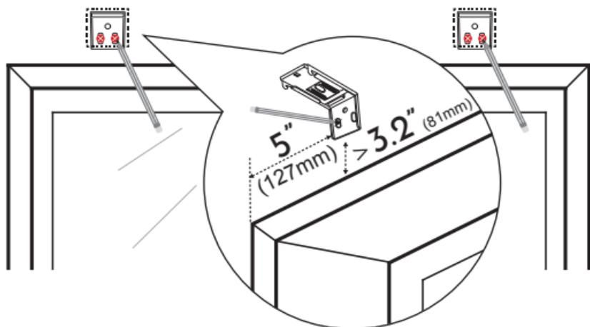
5 Drill holes & install mounting brackets.
