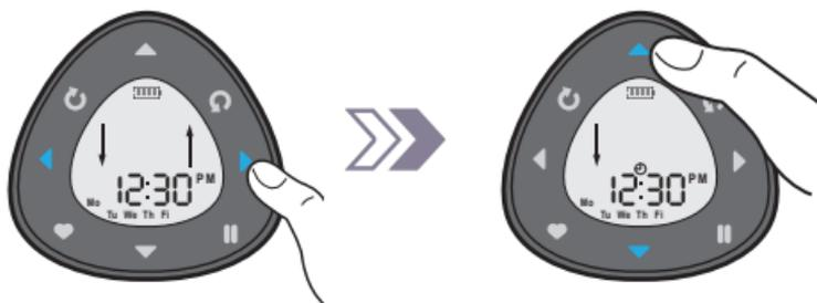
Press "◀" or "▶" to switch between open and close, the selected one will be flashing.
