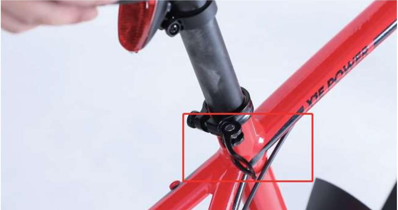
2. Insert the seat post into the frame tube.
