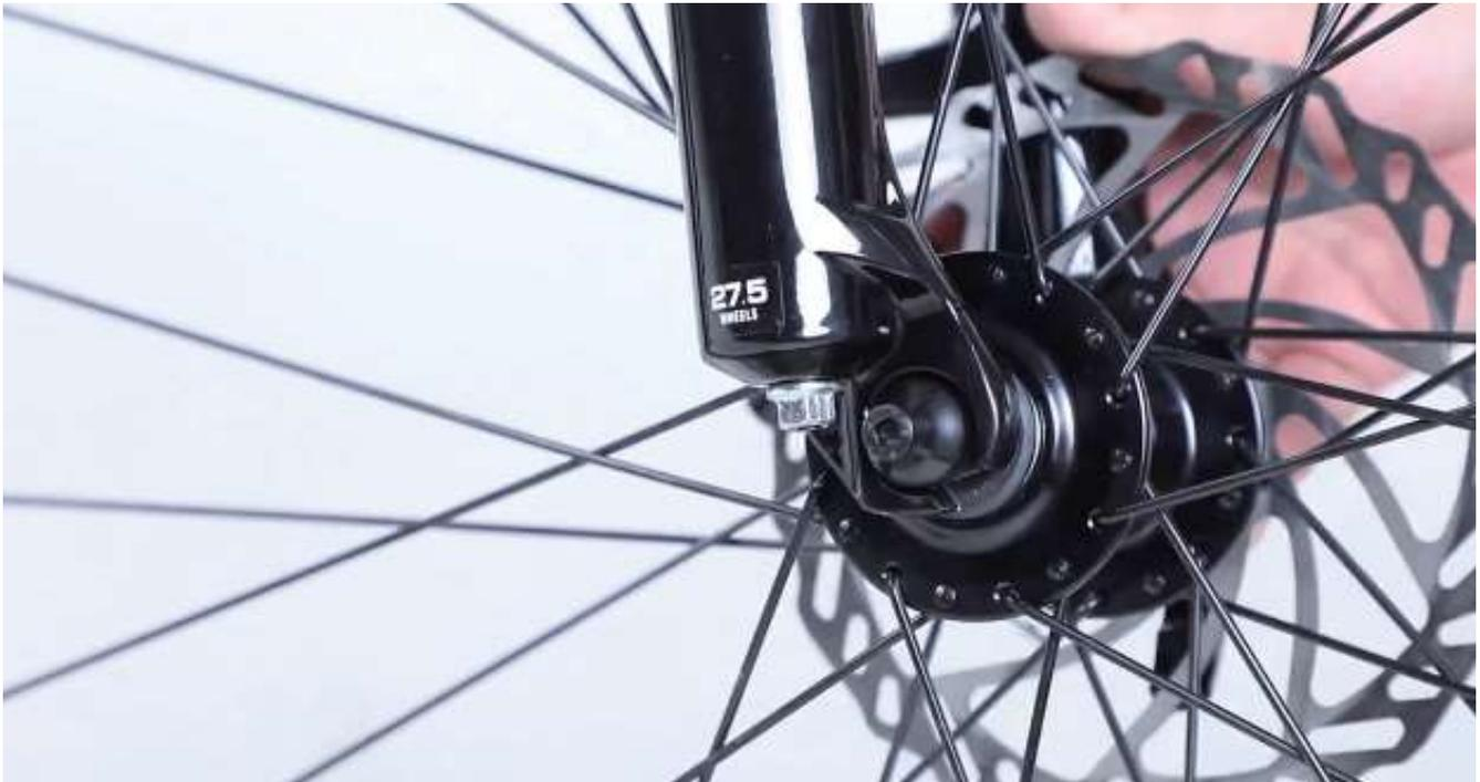
4. Continue to adjust the quick release and nut until they are locked.
