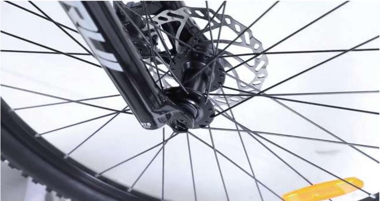
2. Insert the quick release into the hub, note that only one spring on each side.
