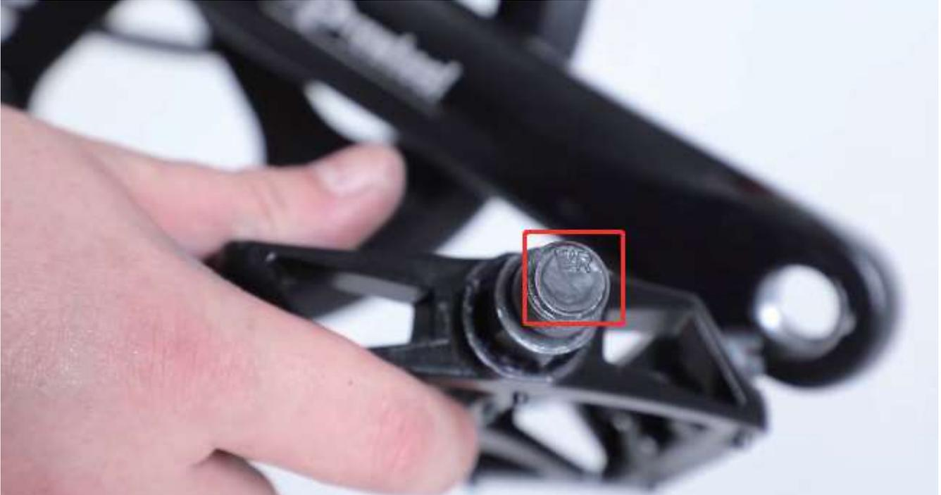
2. Install the right pedal on the right crankset and rotate it **CLOCKWISE** to tighten. (Counterclockwise for the left pedal)
