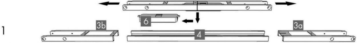
Lay out all components and hardware to ensure that you have all the components and hardware listed on the parts page. Slide the Control Box (part 6) off the Frame End-CB (part 3a) and set aside. Fully separate Frame End (part 3b) from Frame End-CB (part 3a). You will find the Center Rails (part 4) inside.
