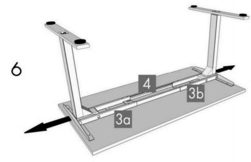
Your desktop may or may not be pre-drilled. Check both sides of the desktop before placing the desk base on the underside of the desktop.
