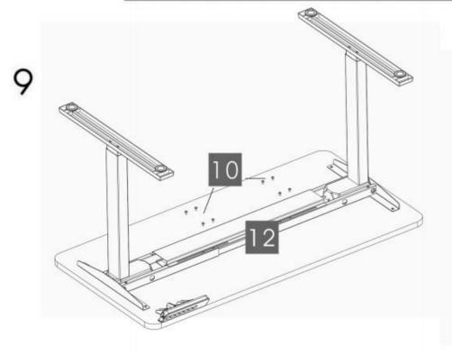
Put the Cable Cover(part 12) into the frame, fixed them with eight M6x10 Machine Screws(part 10).
