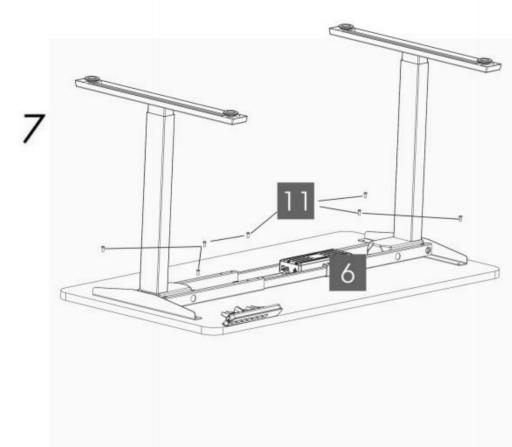
Double-check that the wood screws are not too long for your desktop and won't puncture the surface when screwed all the way in.
