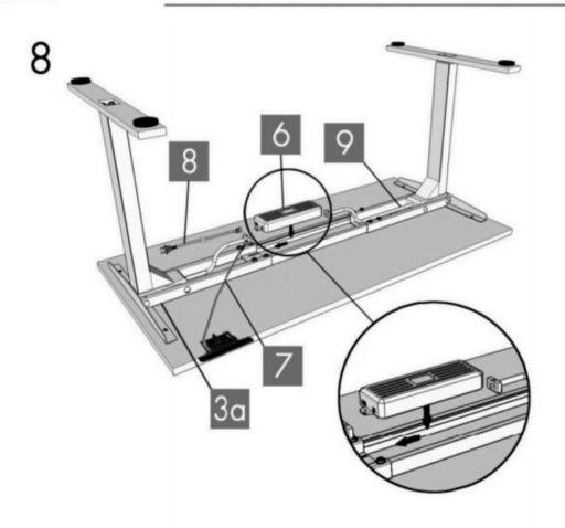
Slide the Control Box (part 6) onto the Frame End-CB (part 3a).
