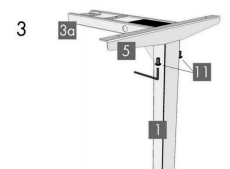
The Frame End-CB (part 3a) should be placed on the side of the desk where you plan to mount the Control Box (part 6) and the Handset (part 7).
