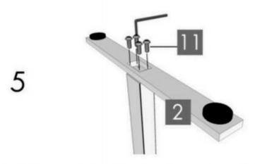
For each leg assembly, attach a Foot (part 2) with four (4) M6x14 Machine Screws (part 11) and tighten in a cross-pattern.
