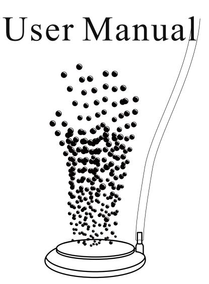
This Series Aquarium air stone is made of high-quality white alundum, be sintered at a high temperature of 1300 degrees Celsius. Its heavy, Sturdy, Durable.
