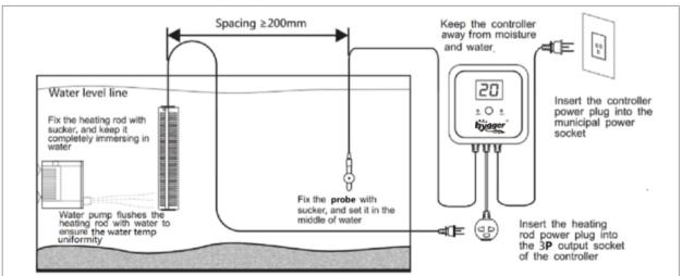
**B.**Press the "SET" button at a time, then the digital screen flashing, meanwhile the red indicator and green indicator is on. Press the "SET" button until reach your desired temperature value and waiting for 5S, then the digital screen shows water temperature, your setting is done. You can press the "SET" button persistently to display 63~93°F in a cycle.
