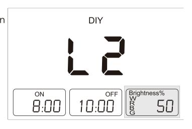
And so on to finish setting L7. The start time of L8 is the end time of L7, and the end time of L8 is one minute before the start time of L1, please note that L1-L8 must be set for the whole 24 hours in DIY mode.
