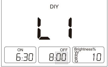
Then press DIY, Brightness flashing you can press WHITE RED GREEN BLUE to increase or decrease the brightness of four colors.
