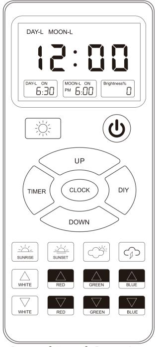
RF Remote Controller: suitable for receiving and transmitting signals at a distance in 10 meters, and can be remote controlled through the wall.
