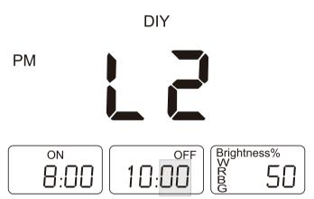
(6) Press DIY , the brightness flash then you can press WHITE RED GREEN BLUE to increase or decrease the brightness of four colors . Repeat the flow above to set L3-L7.
