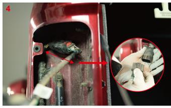
**Notice:** Before you take out the BLIS, please mark the left and right sides of the BLIS plug. During installation, Please pay attention to the installation direction of BLIS and the new taillight. To avoid errors in the subsequent installation steps that may result in non-use.
