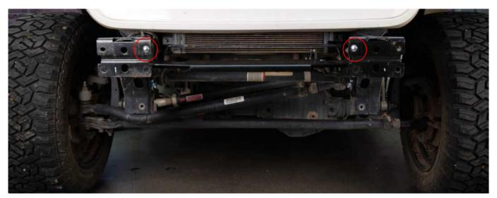
**Note:** The Bolt is only used to fix the Winch Bracket, and it is convenient to install the two mounting holes under the winch bracket. Please Keep it and use it in the next step.
