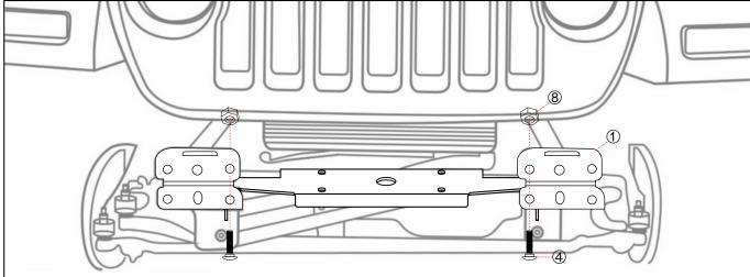
Note: Please mounting the corresponding bolts at the first. Do not tighten the bolt in this step. JK model do not need to use the ③Plate.
