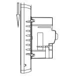
3.Install the fixed plate of thermostat in electrical connection box with screws.
