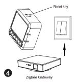
After the wiring of switch module is done, press the reset key for about 10 seconds or Press traditional dimmer off(Either one connected to the wi- dimmer module). Then press and hold for 10 seconds until light connected to the module will quickly and enter into configuration mode or until the indicator light inside the module is flashing quickly for pairing.
