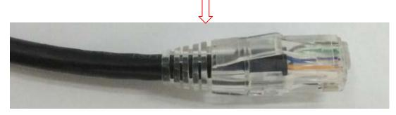
**Step 6:** Use the crimp tool to press the plug and the hook connector
