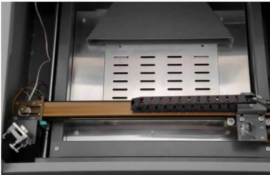
**Fig. 5-3 The second Mirror in Position B**
