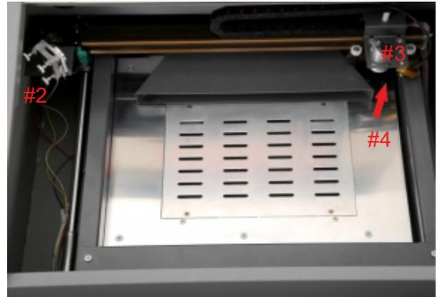
**Fig. 1-2 Mirrors #2-3 & Focus Lens**
