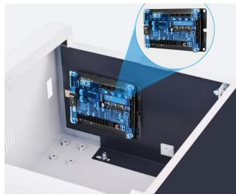
**Step 2:** Connect power supply to the control board.
