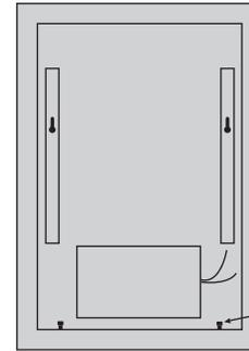
1. Before hanging the mirror on the wall. Locate the secure Screws at the back bottom of the mirror frame, loosen the screws by turning the knobs.
