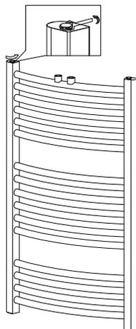
**Step 2:** Securely screw the heating element onto the radiator by spanner (clockwise).
