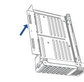
3. Insert the 3.5-inch hard disk, align it with the 4. Place the hard disk in the box with securing columns on both sides, and lock the the tray. hard disk.
