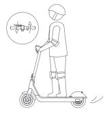
4. Release the accelerator and the kinetic energy recovery system (KERS) initiates automatically to brake slowly; And squeeze the brake lever for a sudden brake.
