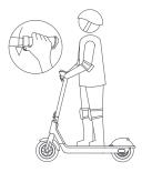
3. When the scooter starts to coast, put both feet on the deck and press the accelerator (the accelerator initiates once the coasting speed exceeds 2.4 MPH).
