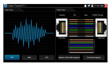
**Note:** if use BNC adapters and alligator clip cable to connect BNC cable etc. Please switch to "BNC mode", if connect shielded cable, please select "STP mode".
