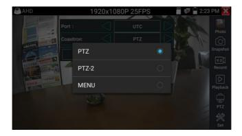
If to coaxial PTZ control the AHD camera, no parameters setting is needed.
