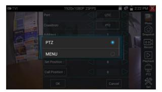
Input calling dome camera menu address code, after finishing the parameter settings, you can press the key "Enter" or click the icon to call the dome camera menu.
