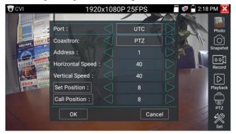
The PTZ address in the tester must be consistent with the dome camera or decoder, then the IPC tester can test. After setting the parameter, the tester can control the PTZ and lens.
