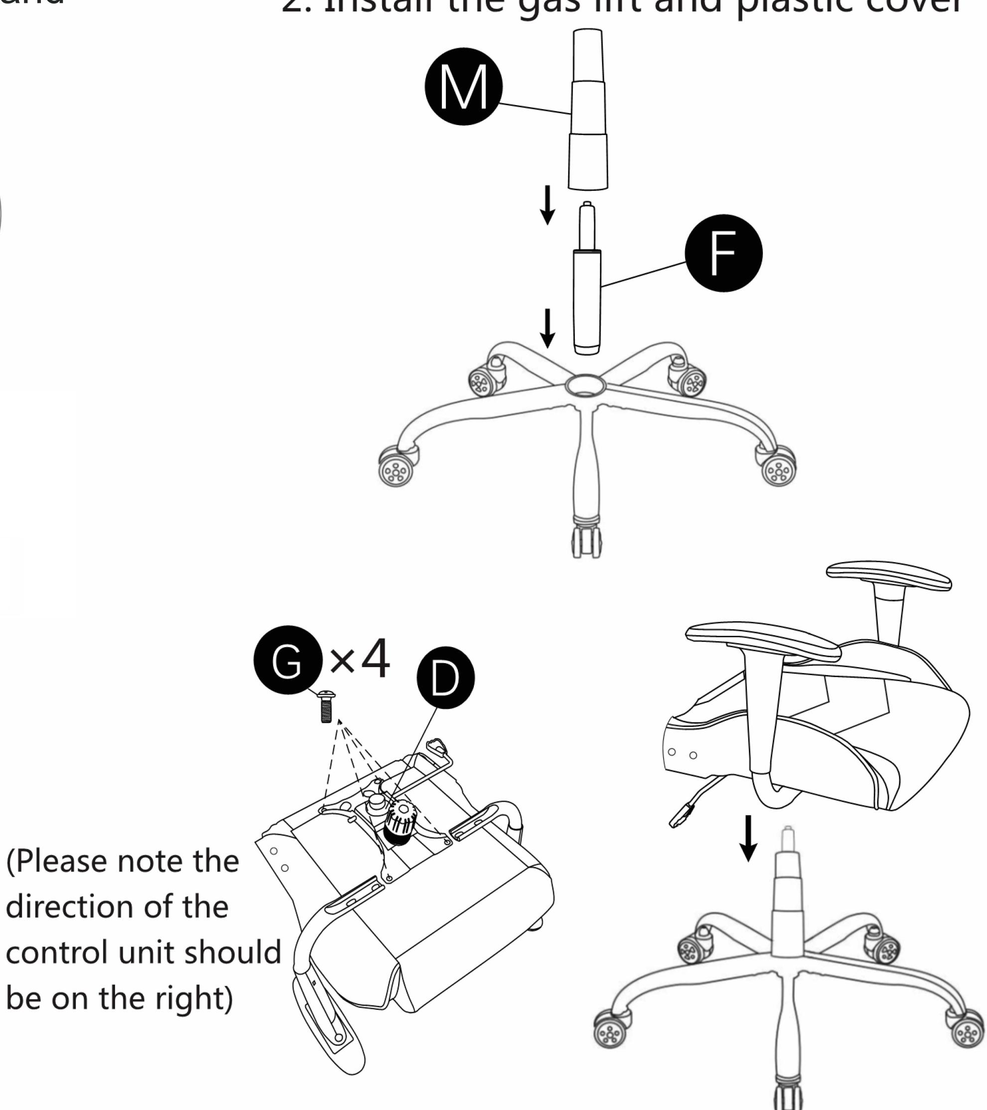
4. Fix the control unit to the base of the seat
