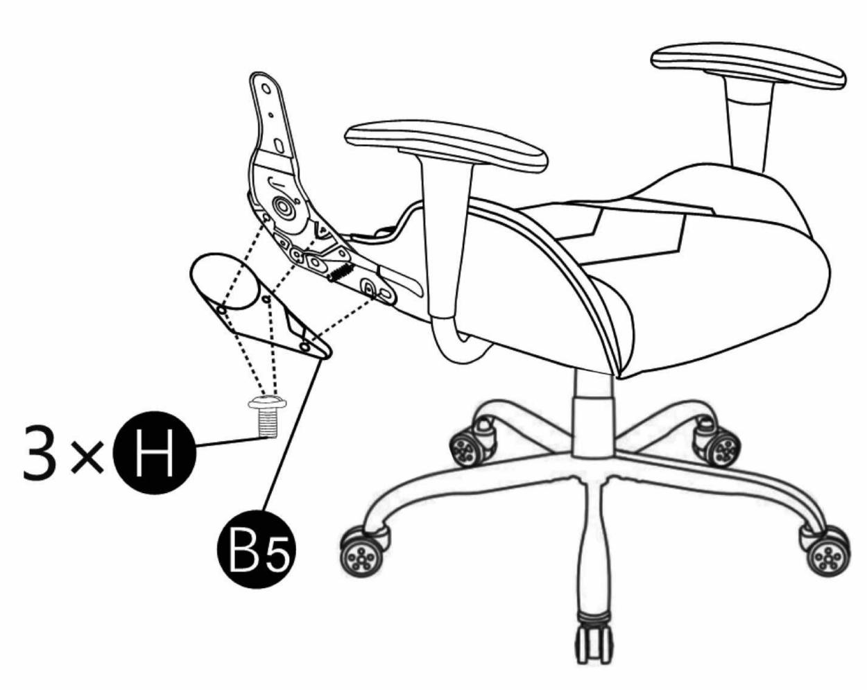
8. Fix the plastic cover(B5) onto the side of backrest
