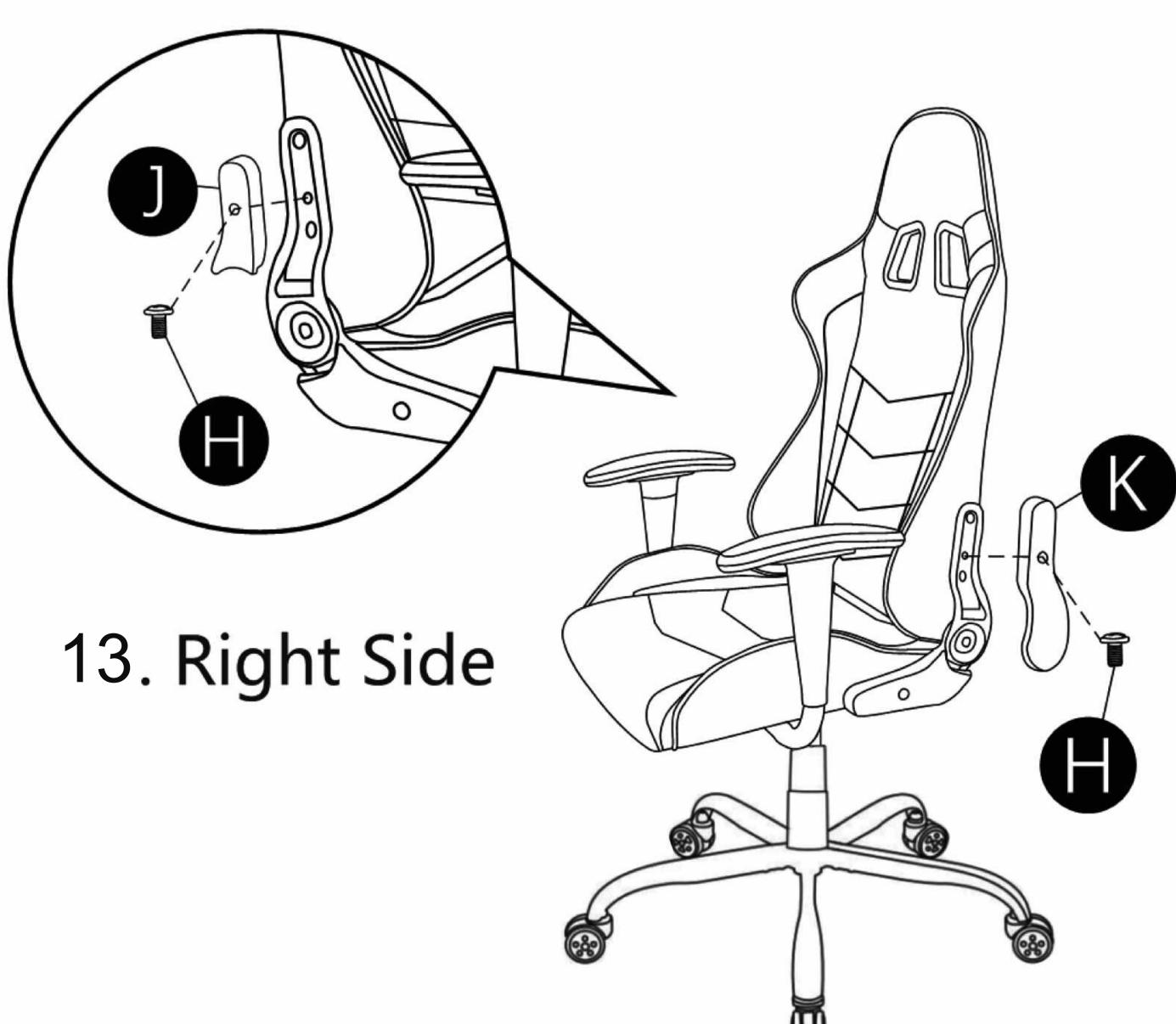
12. Fix the plastic cover(K) onto the side of backrest
