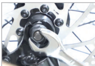
Both sides must be tightened
