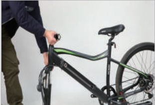
Put the handlebar on the stem
