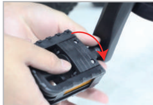
Installed on the chainwheel side crank
