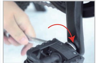
Rotate clockwise to tighten
