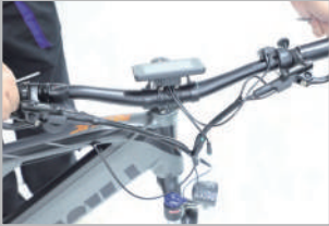
Put the handlebar on the stem
